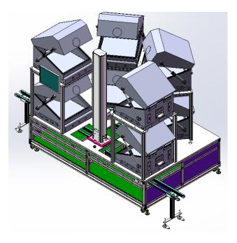
Also if the shielding box is too big to be placed as two-layer structure, we can install the 5<sup>th</sup> axis of robotic arms. It enables the robotic arm to move horizontally to pick DUT from many shielding boxes.
